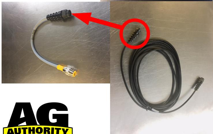
Plug in the AgCam camera cable into the other end of the extension cable and the other end of the camera cable into the back of the camera.
