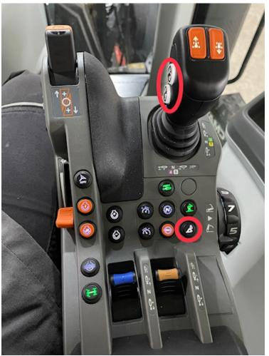
Press and hold the bucket lock button and either the F3 or F4 button together. Then press Either F1 or F2 at the same time To unlock and lock the bucket. Three buttons will need to be held down at the same time. The bucket will pivot at the same time when F1 or F2 is pressed.
