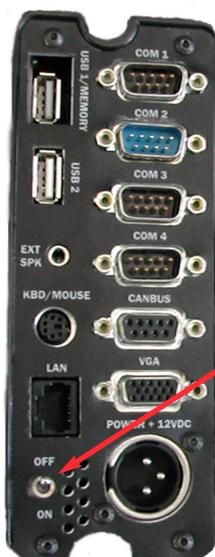
3. Press and hold down the Power Switch for 1 second to turn console ON.
