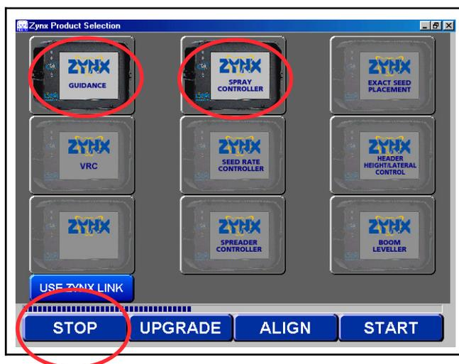
Selection of the products is done at start up on the Startup screen, as shown. Select "STOP", to allow time, to make a selection change.
