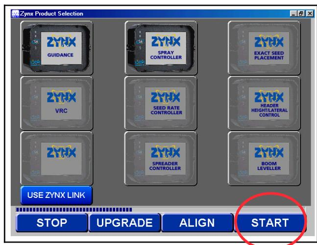
Once the modes are selected press "START" and the corresponding ZYNX solution will be ready for operation.
