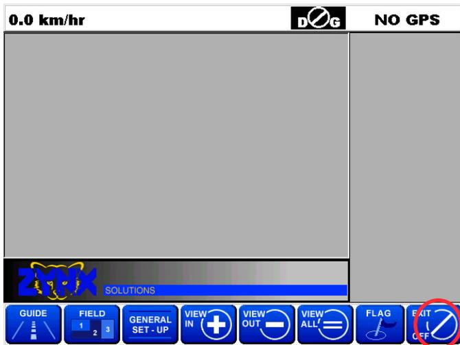
To return from a ZYNX Solution (Guidance is shown here) simply touch the "EXIT" button.
