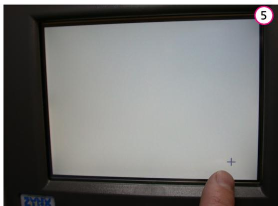
Once the screen cross-hairs have been touched 5 times, the screen automatically returns to the ZYNX Startup screens.
