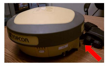
3) Last you will need to hold down the white function button and restore the main cable back to the AGI3. Note, you cannot let up on the white Function button until you see the LED's blink through the series of blink explained below.
