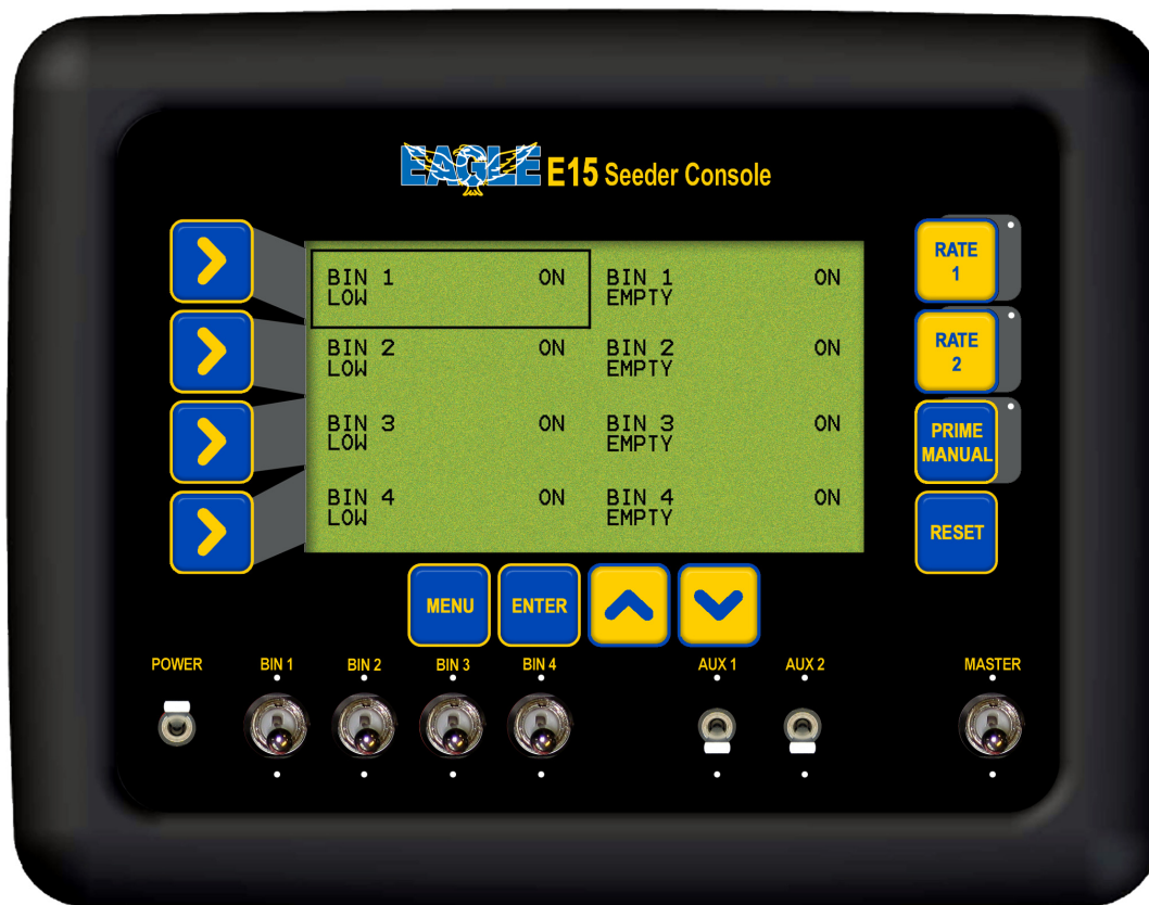
Bin Alarm Screen
