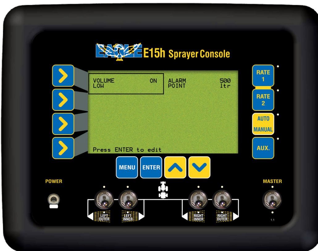
Tank Alarms Screen
