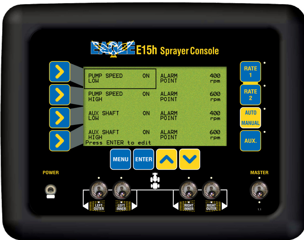
Shaft Alarms Screen
