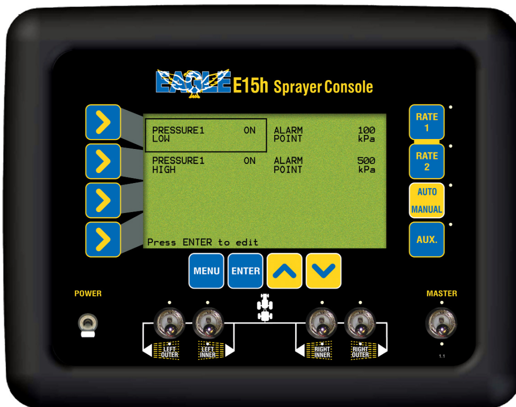
Pressure Alarms Screen
