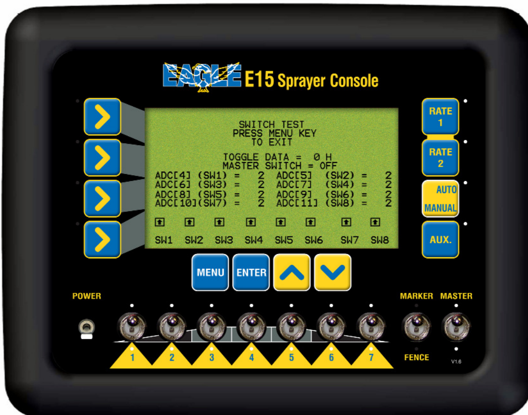
Switch Diagnostics Screen
