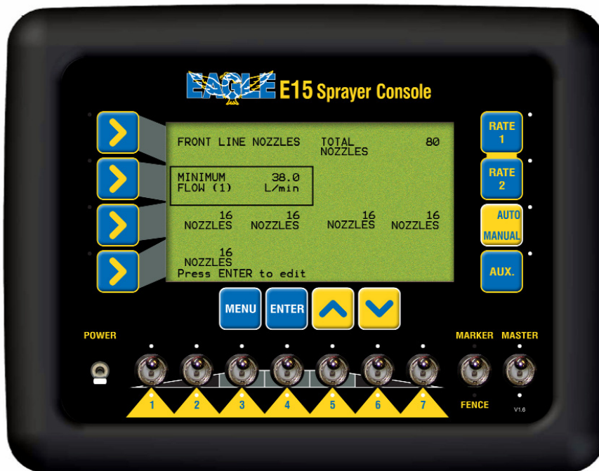
Front Line Nozzles screen
