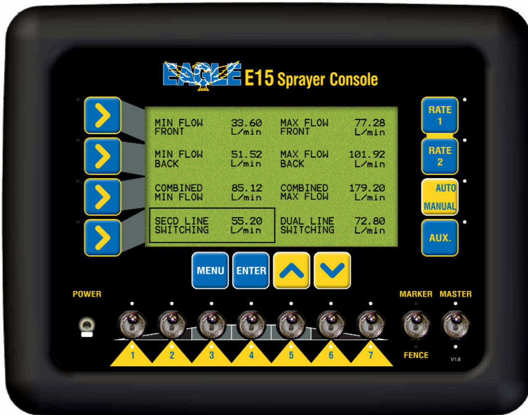
Dual Line Switching(Flow) Screen
