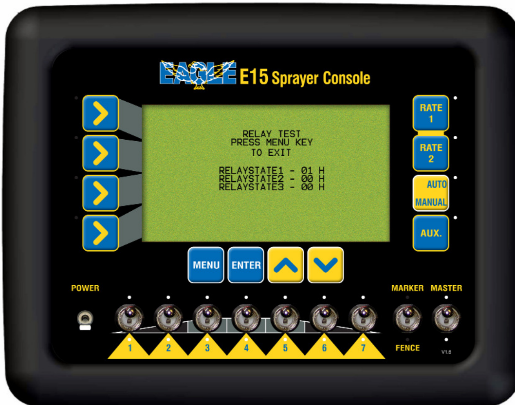
Relays Diagnostics Screen
