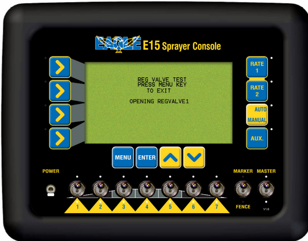
REGULATOR Valve Diagnostics Screen
