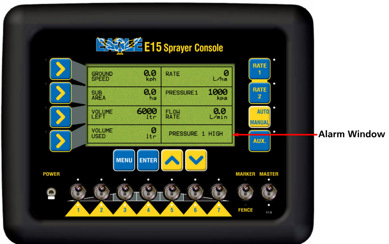
Working Screen showing Alarm
