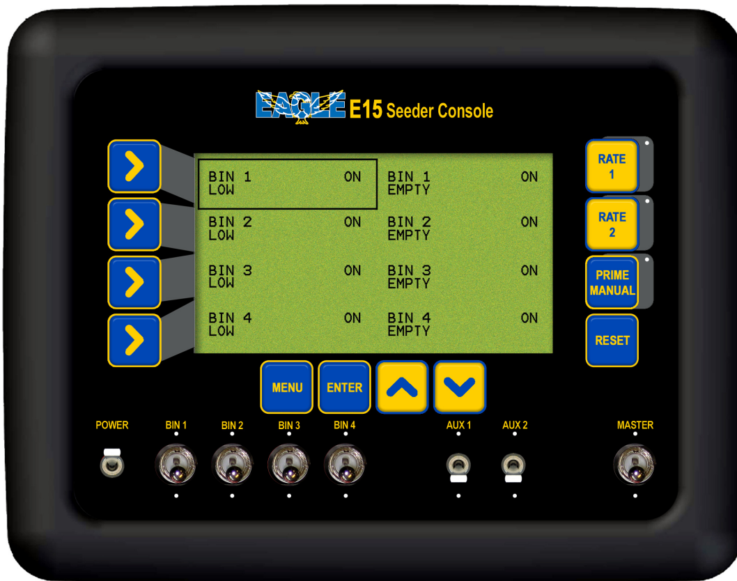
Bin Alarm Screen
