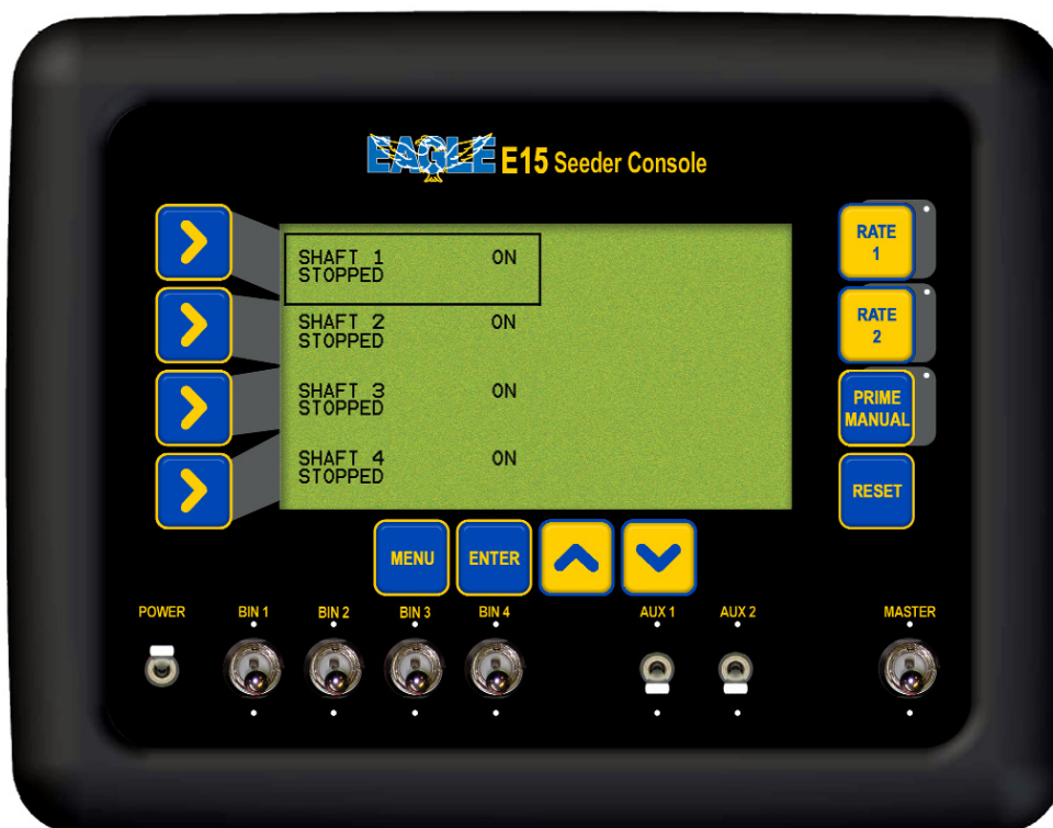
Shaft Alarm Screen
