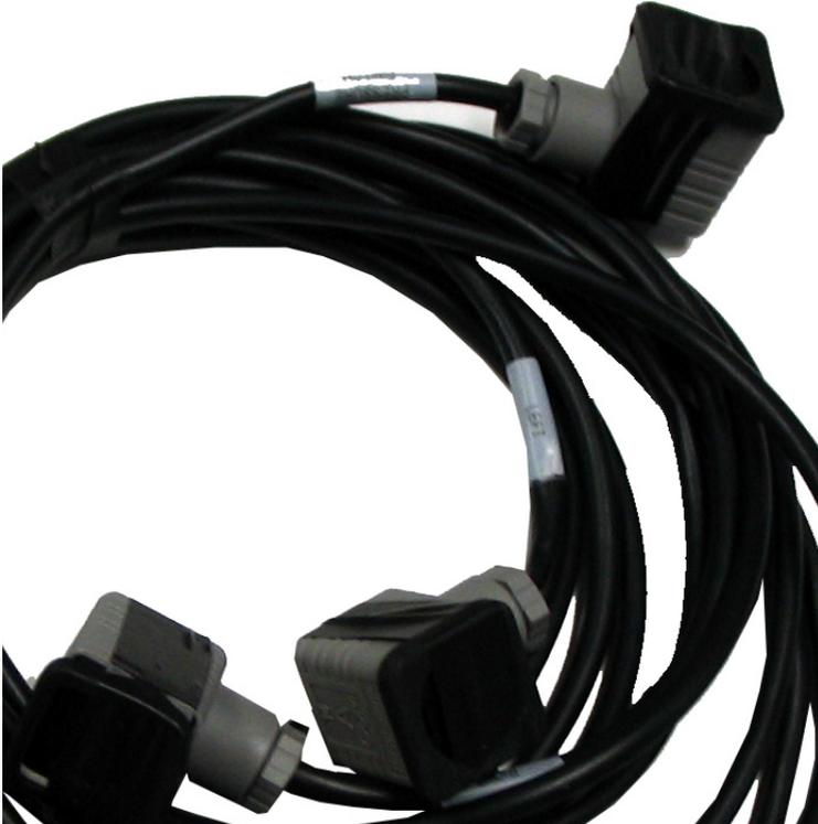
Left and Right proportional valve connectors, fit onto the proportional valve on the Series III hydraulic valve block. If the vehicle turns left (when right is selected) when testing within procal, simply swap the proportional hirshman connectors over.
