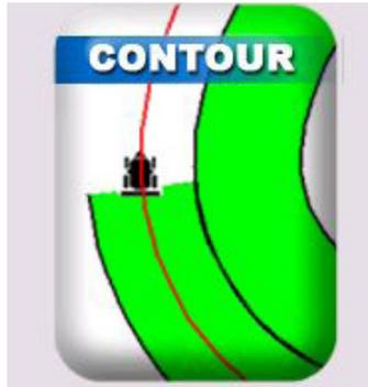
To utilise this function (adjust steering performance of contour), firstly set a curved application line. Go to the guidance run time screen and touch the tractor icon. This will start “painting” an application map in green when the vehicle is moving.
