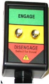
Engage: Momentary switch, that is used to engage the steering. Push the switch up, it will engage the Auto Steering and return to the centre position
