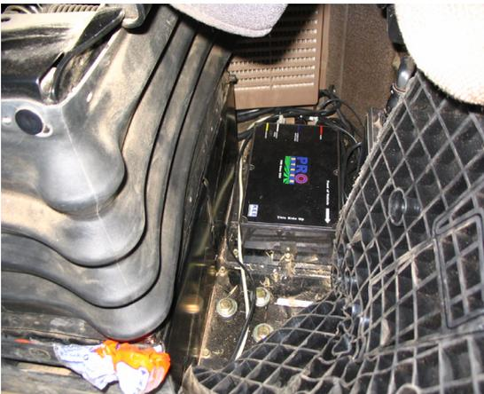
Showing the ECU mounted to the floor on the left hand side of the seat (as you sit in the seat), on a JD 7920 FWA tractor
