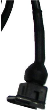
There are two Bosch connectors that fit to the isolation valves on the Series III hydraulic valve block. It does not matter which isolation valve cartridge they fit, as they are wired in series.
