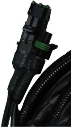
In Cab power connection. (only to be used if the power cable cannot be connected to the hydraulic harness)
