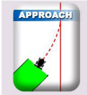
To utilise this function (adjust steering approach to the line), firstly set a parallel line. Set point A, drive at least 20m (60 yards) and then select point B, and then PARALLEL.
