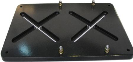
The ECU is supplied with a Quick Mount Plate (A2907) for ease of moving the ECU from one vehicle to another. It is also provided to so that the ECU has a stable mounting surface so that it is unable to move, and thus allowing the tilt/gyro sensors to work effectively. Failure to secure the ECU correctly will result in poor steering performance.
