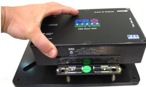
Once the Quick Mount is securely installed, place the ECU over the locating poles.
