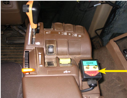
Showing the Switch-box mounted onto the tractor console.
