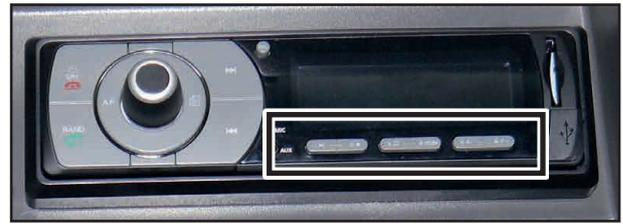
In radio mode, stations can be stored here. In media mode (USB or SD card), playback can be controlled here.
