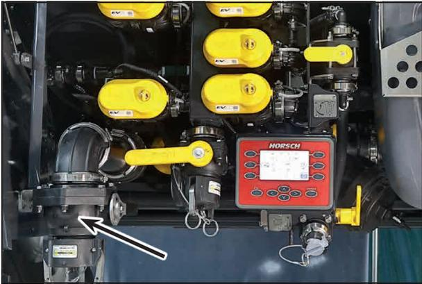
Residue drain of water systems Basic Pro and CCS Pro
