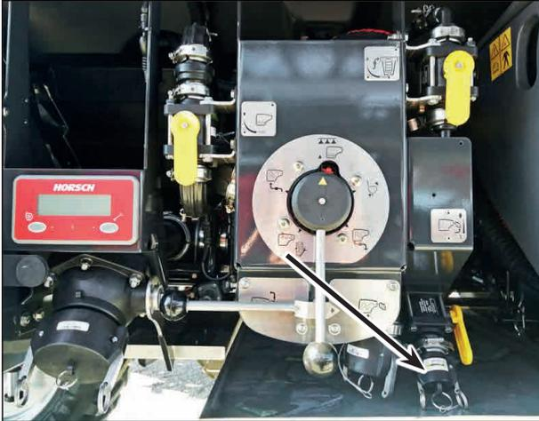
Port for water systems Basic and CCS fresh water tank
