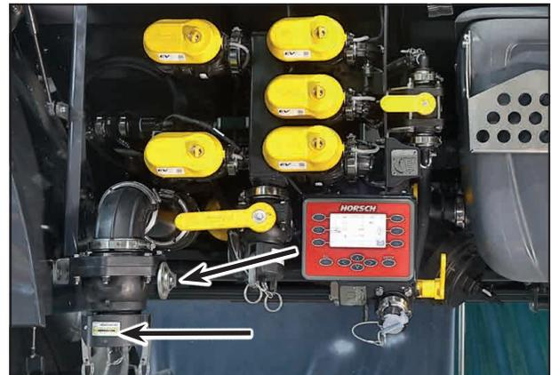
Filling port for spraying mixture container
