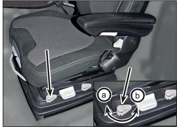
Under certain operating conditions it is advantageous to switch on the horizontal suspension. This enables the driver's seat to better absorb impact loads in the direction of travel.
