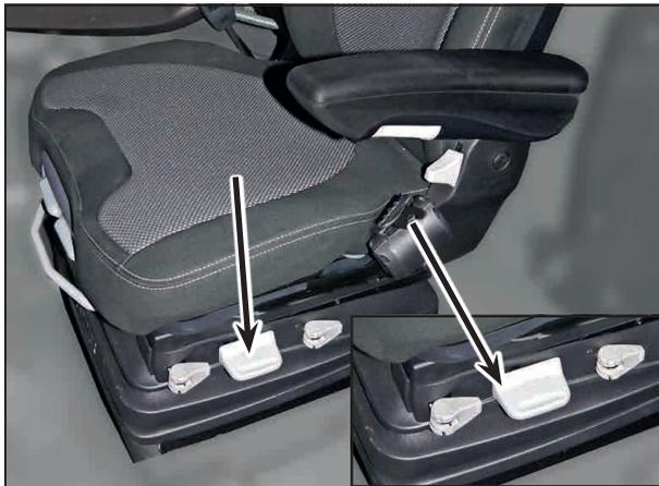
The air-cushioned height adjustment can be infinitely adjusted.
