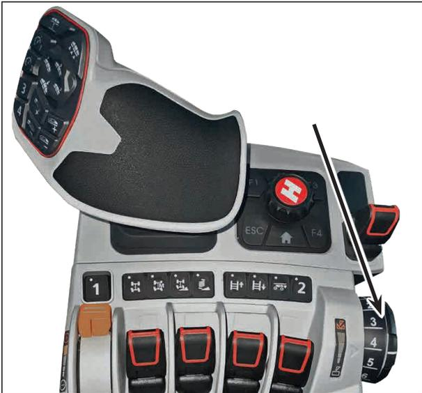
Manual correction for drift on a slope
