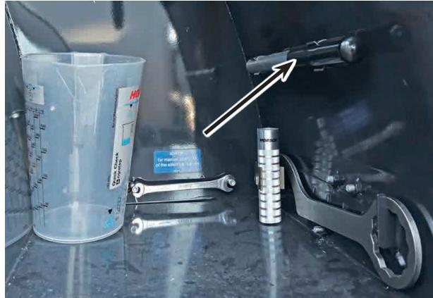
Mechanical release device actuating lever
