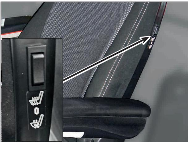
The seat heating is switched on by flipping the switch on the left side of the backrest upward. The seat heating is switched off again by returning the switch to the centre position 0.
