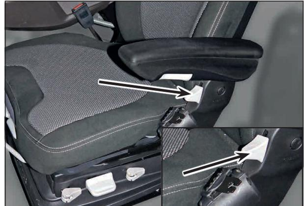
Pull the lever up to adjust the backrest. Do not press against the backrest while unlocking it. The desired position is reached by simultaneously loading and unloading the backrest. Release the lever to lock again.
