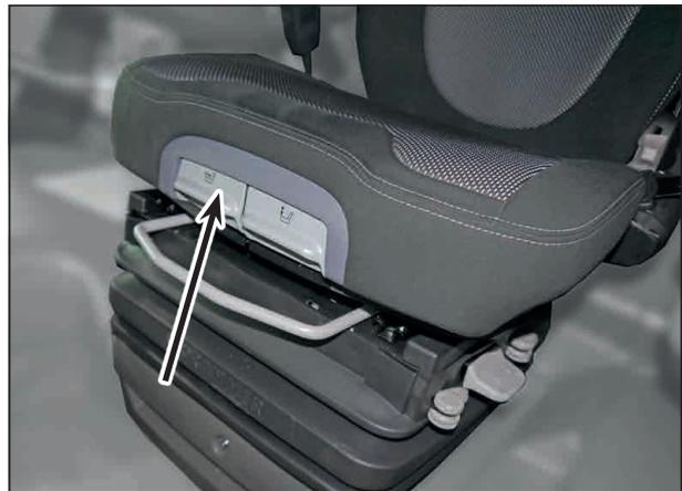
The seat depth can be individually adjusted. Pull the right handle up to adjust the seat depth. The desired position is reached by simultaneously pushing the seat area forward or backward.
