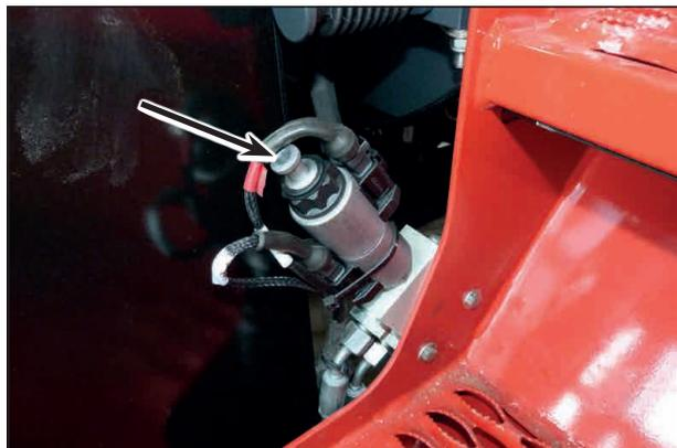
Valve for mechanical release of access ladder
