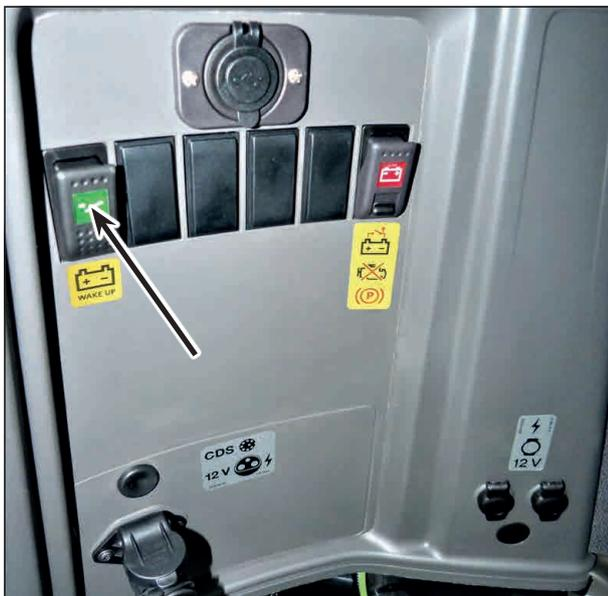
Main battery switch for power supply
