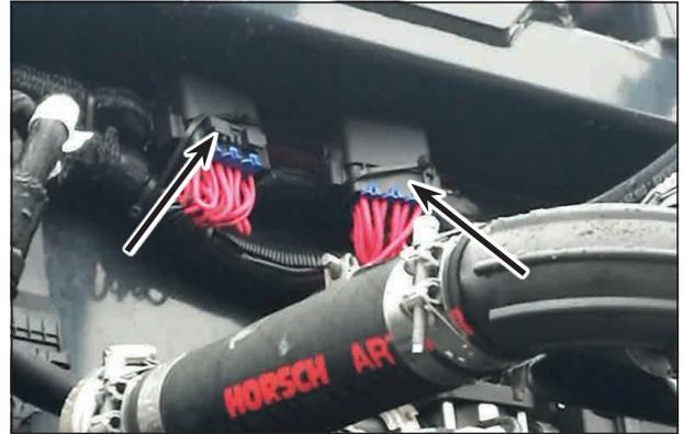
Position of pulse width modulation fuses
