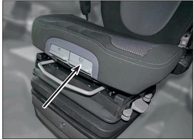
The inclination of the seat area can be individually adjusted.
