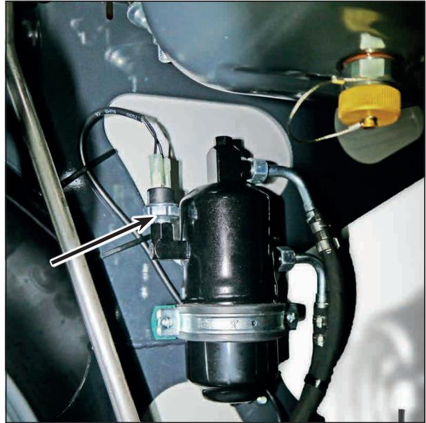
Drier cartridge pressure switch
