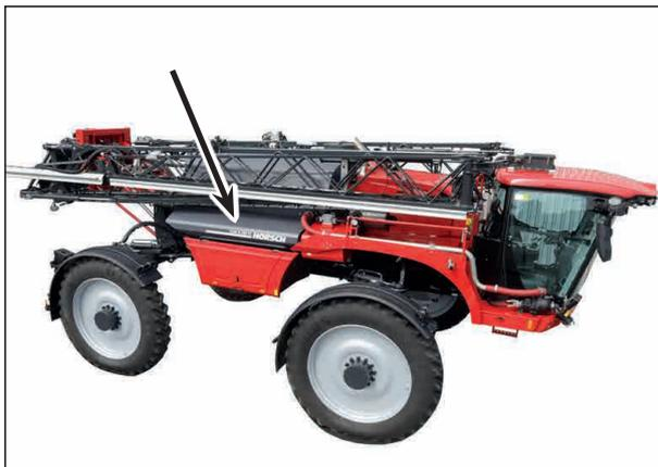
Fresh water tank left and right on the machine
