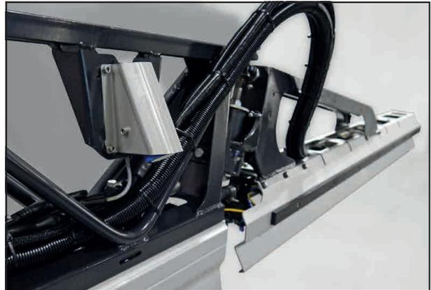
Ultrasonic sensor on the folding boom
