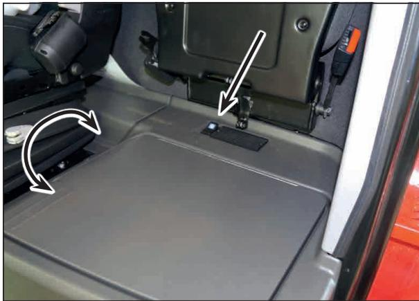
Storage compartment with integrated cooling function under the seat area of the instructor's seat.
