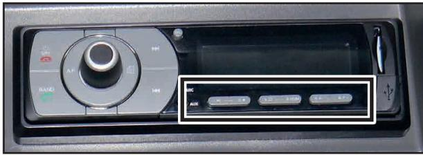
Press and hold one of the preset buttons to store the currently set station. A stored station can be called up by briefly pressing one of the keys. A stored station can be overwritten at any time by setting another station.
