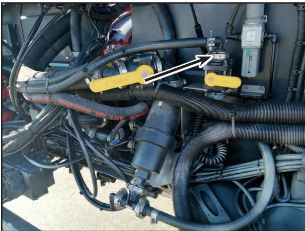
Water separator and filter-regulator combination
