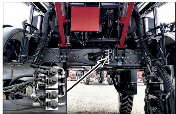
Mechanical release device TrackControl rear axle
