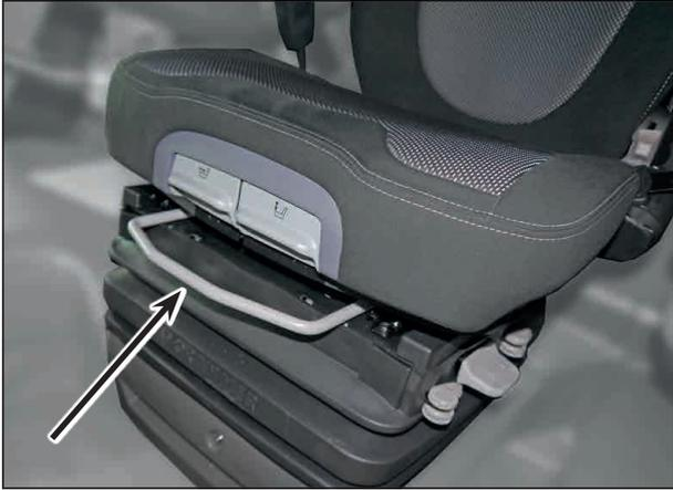
By pulling the operating lever up the longitudinal adjustment is released and the driver's seat can be moved forward or backward.
