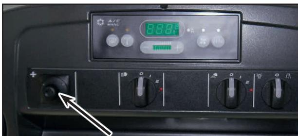
Switch for adjusting the outside mirrors
