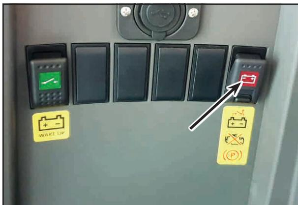
The red switch is used to shut off the current supply early. The battery is disconnected from the vehicle electrical system without overrun time. The diesel engine shuts itself off. The exhaust gas treatment (optional) keeps running for another 15 minutes until final shut-down.
