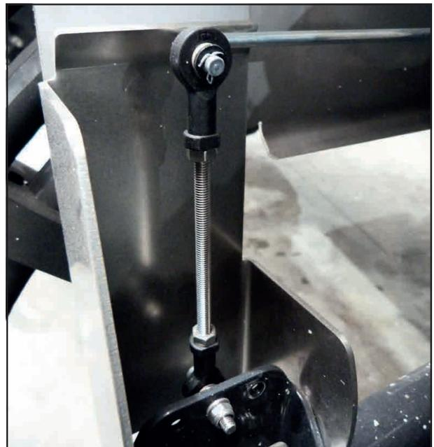
Folding boom level suspension hooked up
