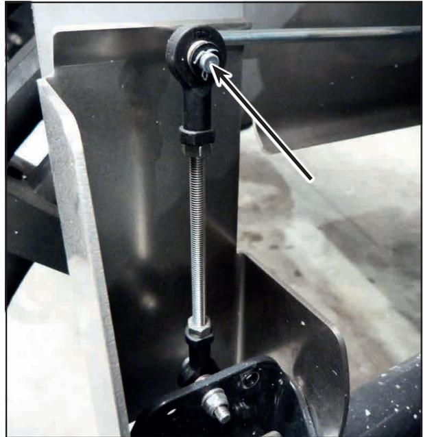
Folding boom level suspension hooked up
