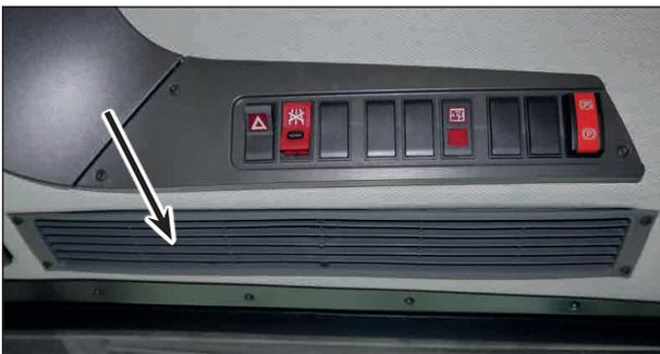
Two additional air recirculation filters are located on the right and left of the roof console above the driver's seat.
