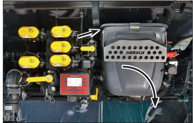
Flush the respective preparation through the illuviation valve into the water of the spraying mixture container. A difference is in this case made between the illuviation of fluid and powdery preparations or carbonyl diamide.
