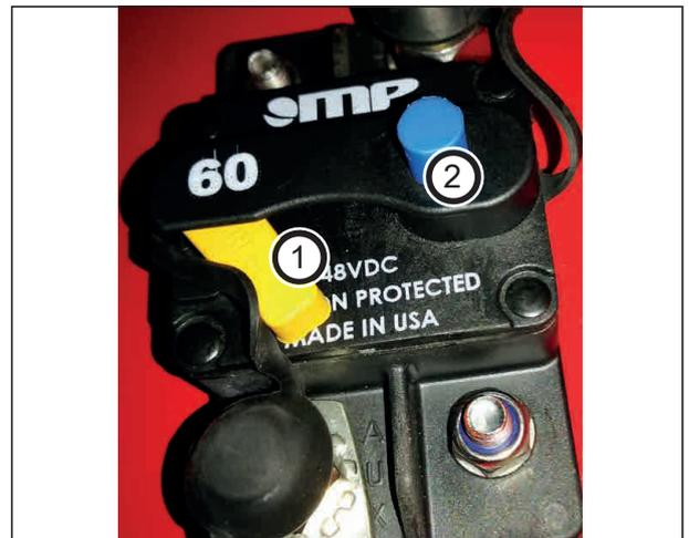
Main fuse PWM nozzles/control unit PrecisionSpray power supply, optional (battery compartment)
