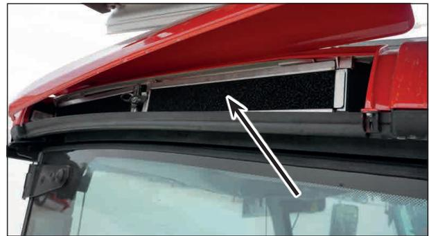
Activated-carbon filter with pocket filter
