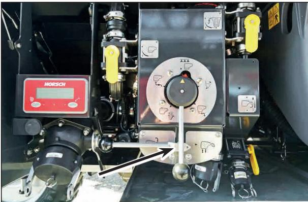
2. Drain the filter housing. Open the valve for this purpose. Collect used fluid and dispose of properly.
