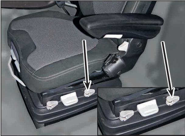
Under certain operating conditions it is advantageous to switch on the lateral horizontal suspension. This enables the driver's seat to better absorb impact loads from the side. The suspension comfort can be switched on and off via the locking handle.
