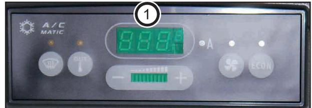
The device then carries out a self-test, which takes a maximum of 20 seconds. The buttons are then enabled for operation.
