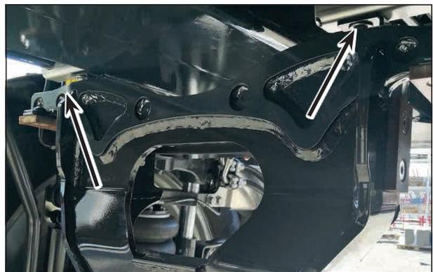
Lifting device with mounting bracket
