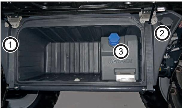
Fuel tank (figure shows the variant with stage V engine and tank for carbonyl diamide solution)
