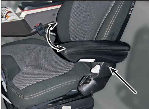
The left arm rest can be folded back and adjusted in height, if required.
