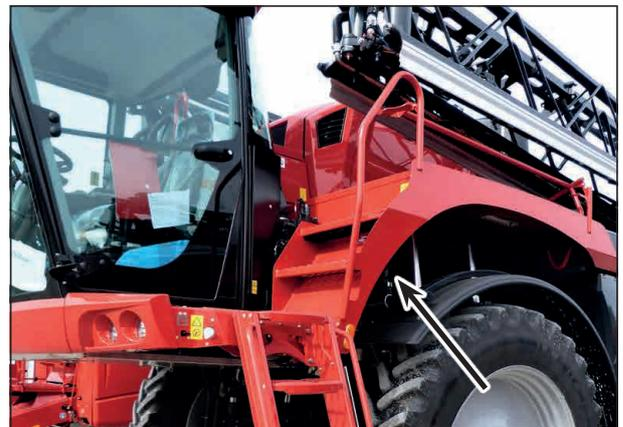
Compressed air system dryer cartridge position
