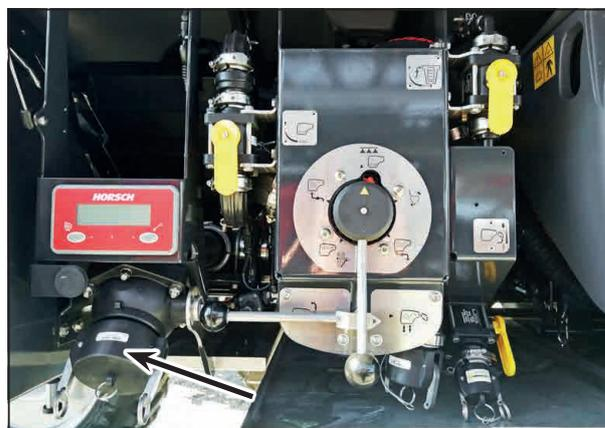
Residue drain of water system Basic and water system CCS
