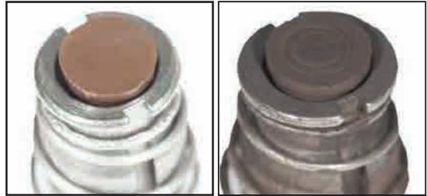
Valve piston (5) new (left), worn (right)
