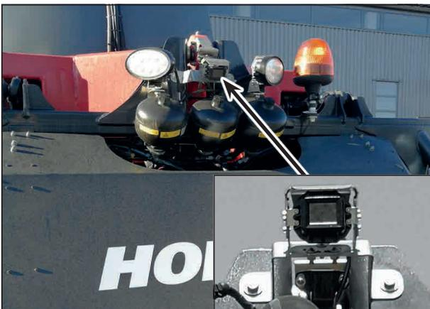
Rear view camera in folding boom middle section
