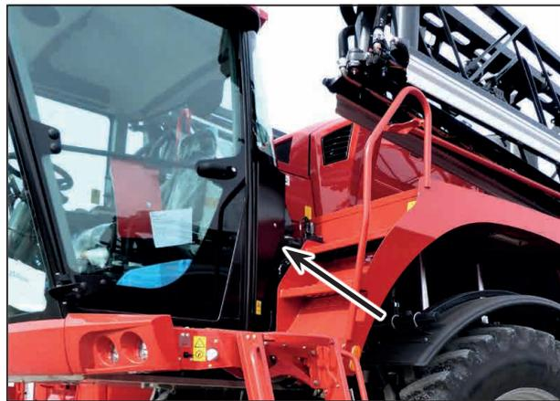
Mechanical release device of access ladder
