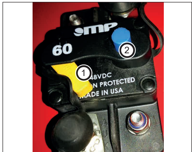
Main fuse Power supply PWM nozzles/control unit PrecisionSpray optional (battery case)
