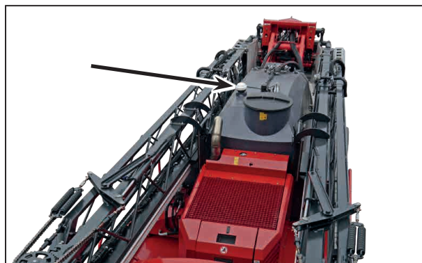
GPS receiver mounted on spraying mixture container
