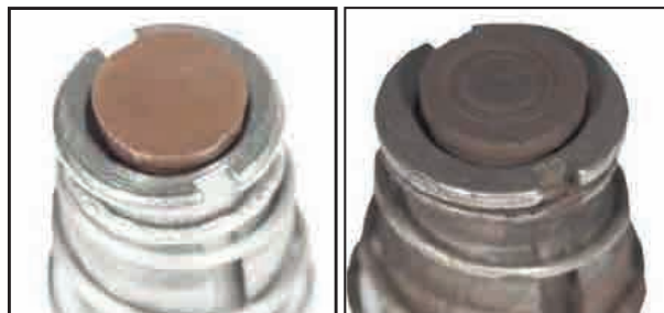
Valve piston (5) new (left), worn (right)
