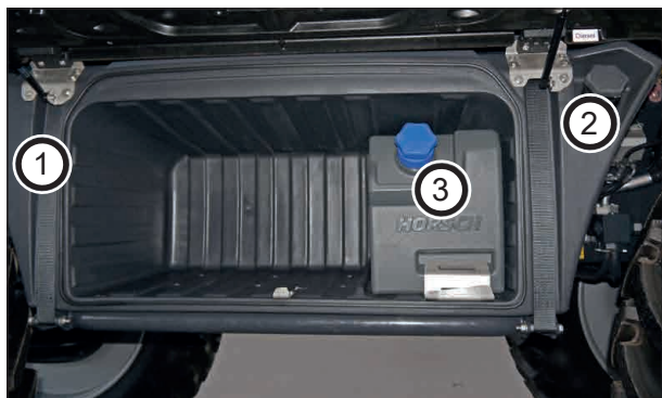
Fuel tank (the figure shows the variant with Stage V engine and AdBlue tank)
